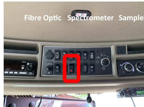
Figure 2.23, Spectrometer Power Switch installation
