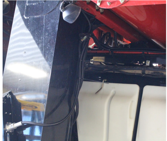
Figure 2.19. Sample Head and Fibre Optic Cable Run.
