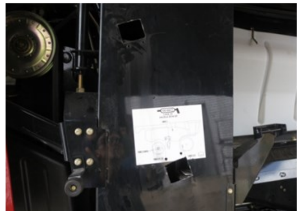
Figure 2.3. Clean grain elevator cut outs.
