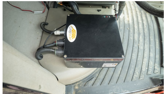
Figure 2.8 NIR Spectrometer Box fitted UCM Panel.
