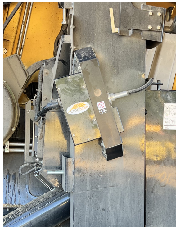
Figure 2.18 CropScan 3300H Sample Fibre Optic Cable.
