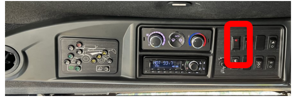
Figure 2.23, Spectrometer Power Switch installation
