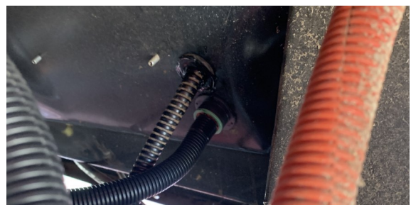
Figure 2.21. Sample Head Cable and Fibre to Cabin.
