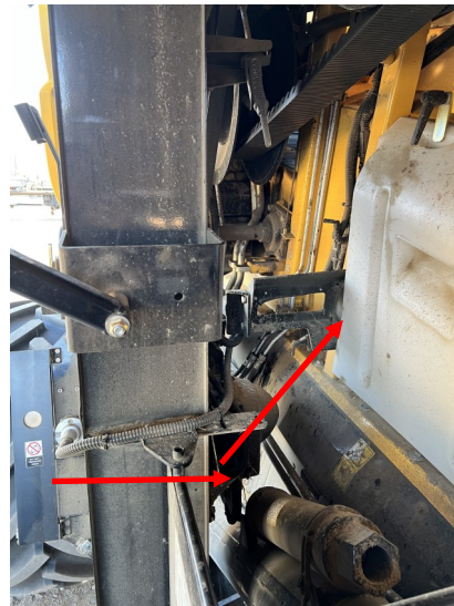
Figure 2.19. Sample Head and Fibre Optic Cable Run.
