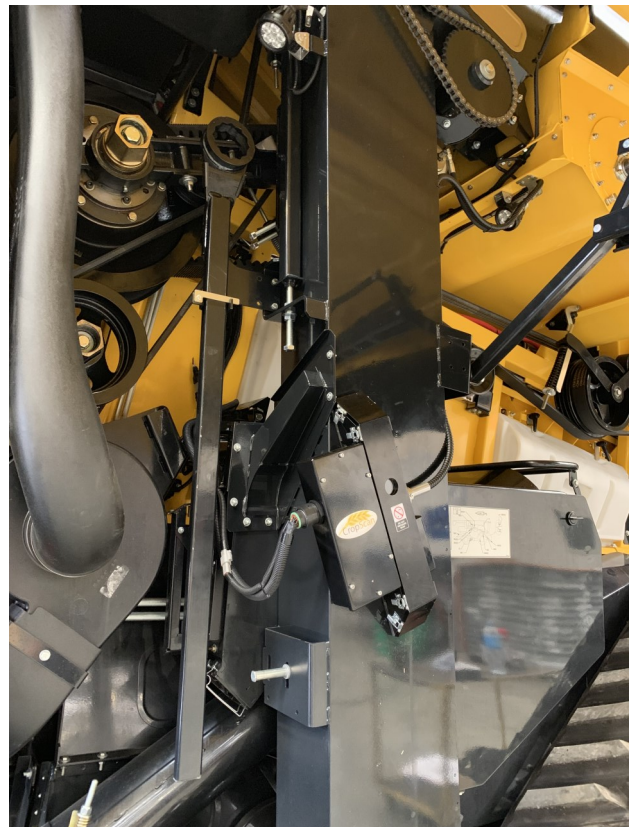
Figure 1.2 Sample Head mounted to the Clean Grain Elevator.
