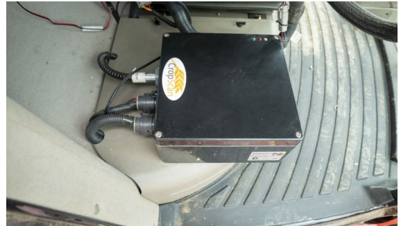
Figure 2.8 NIR Spectrometer Box fitted UCM Panel.
