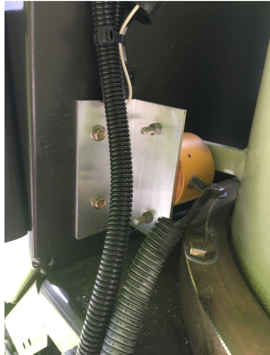
Figure. 2.9. Auger Sensor installation CLAAS Combines.
