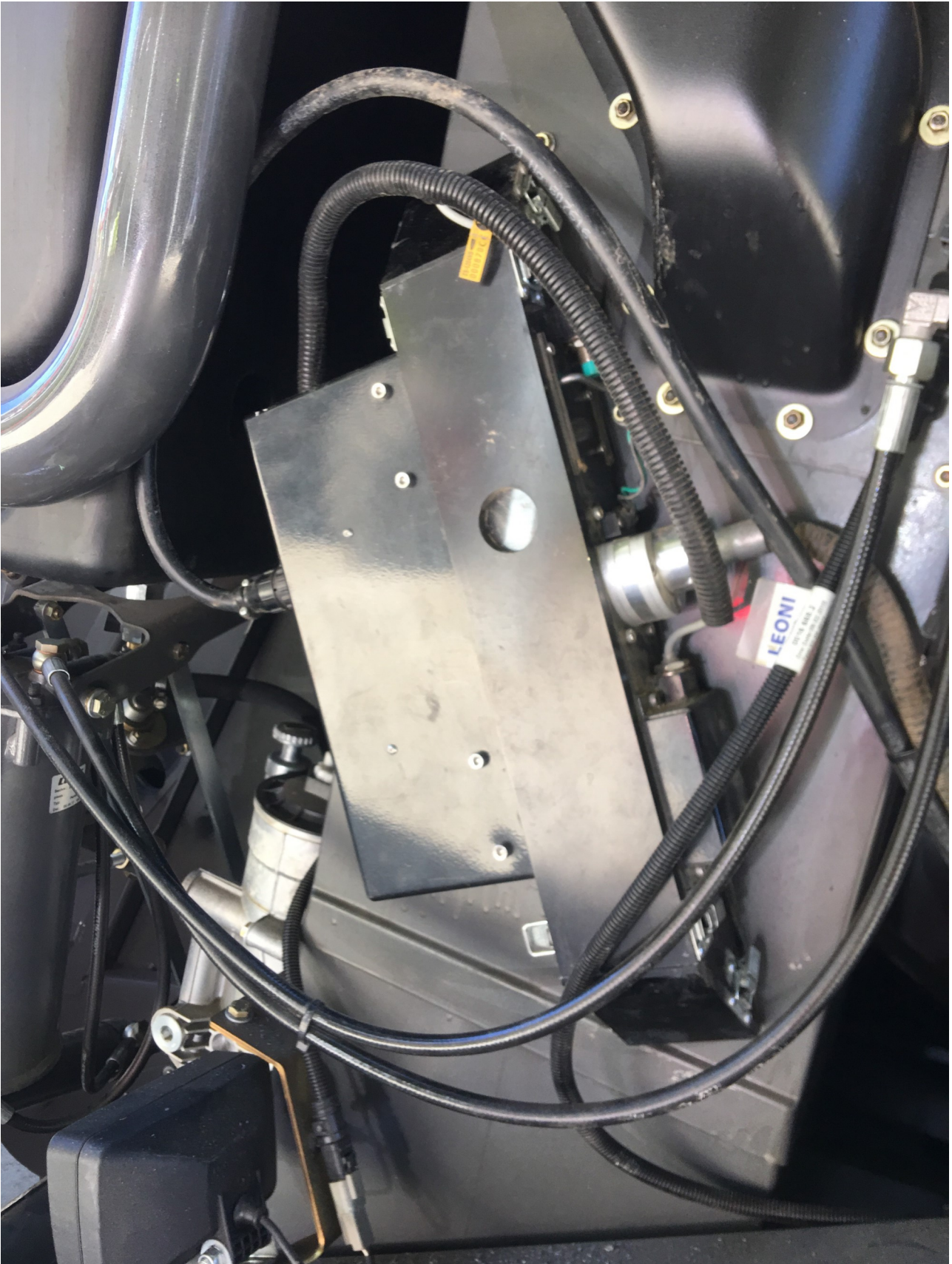
Fig. 5.4. 3300H Remote Sample Head Installation lower elevator position.
