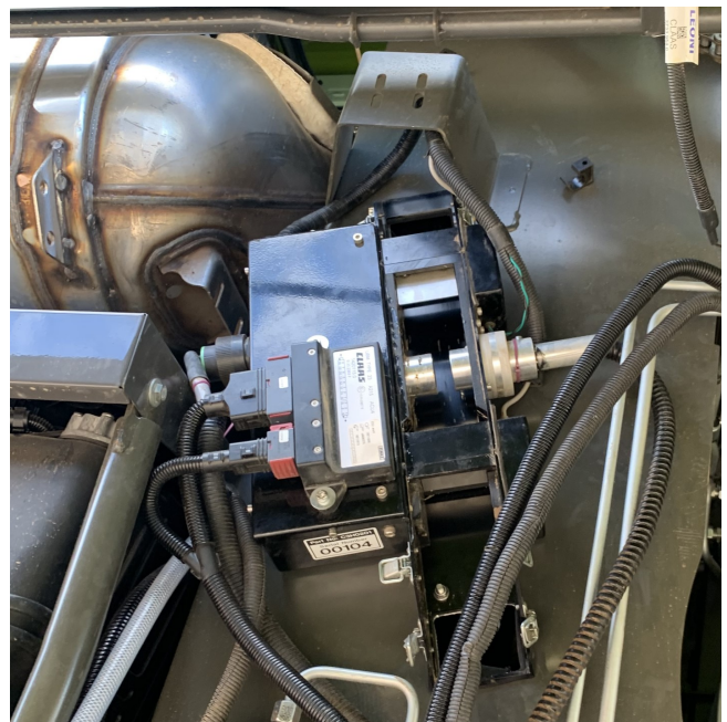
Figure 1.2 Sample Head mounted to the Clean Grain Elevator.
