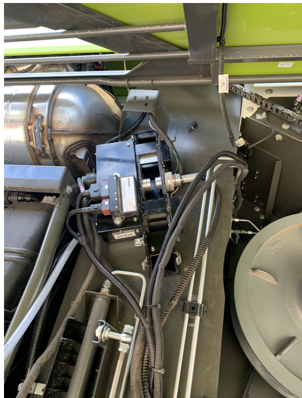
Figure 2.2. Layout for mounting the Remote Sample Head to the Clean Grain Elevator—upper position.
