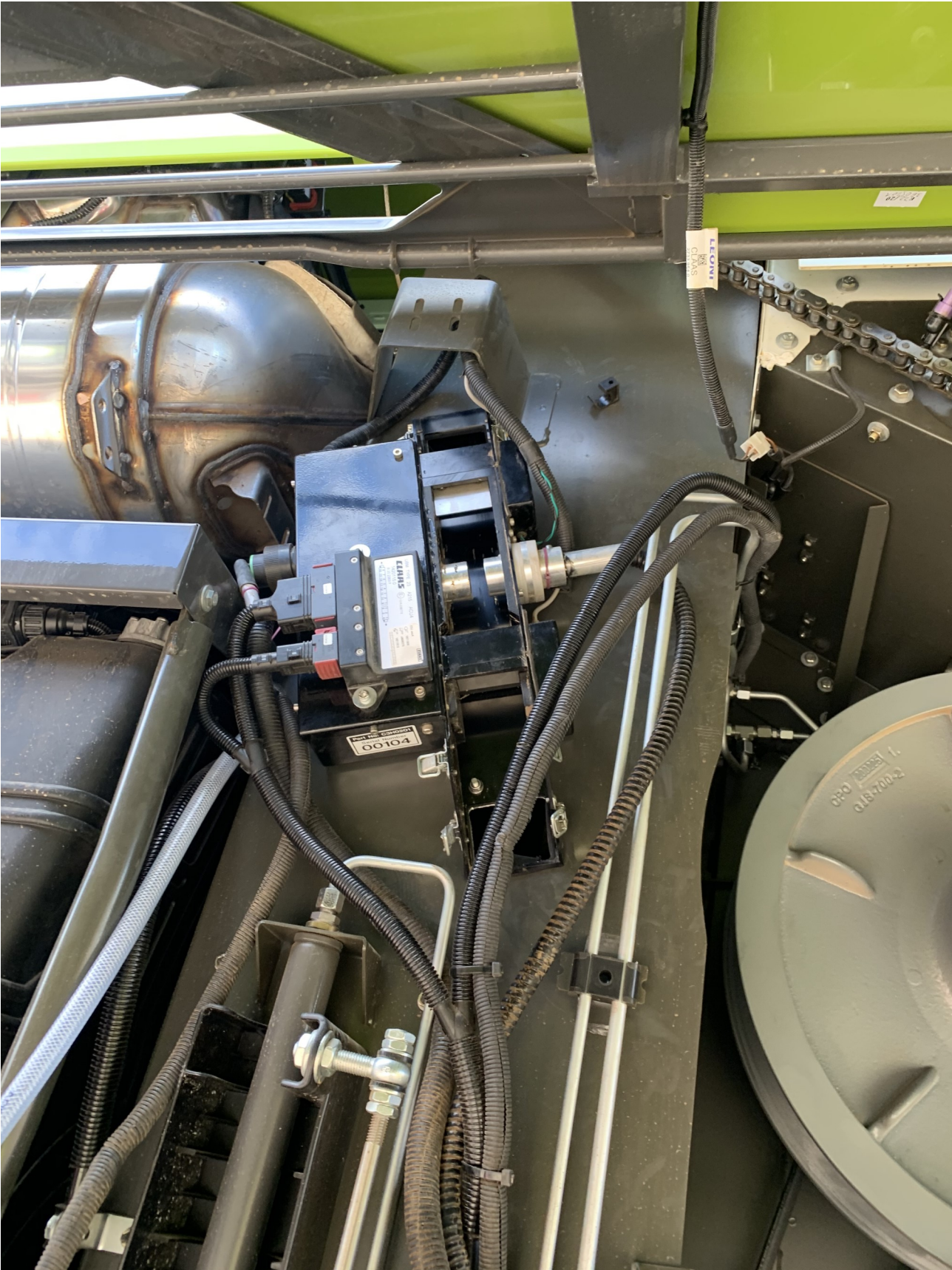
Fig. 5.6. 3300H Remote Sample Head Installation upper elevator position.
