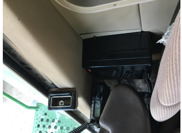
Fig. 2.7. NIR Spectrometer Box fitted to back wall.
