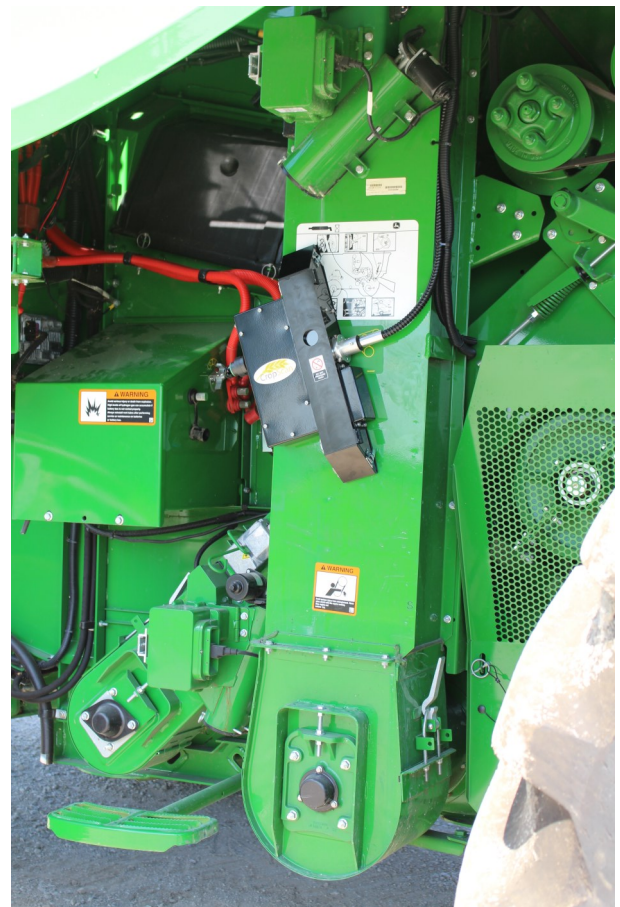
Fig. 1.2 Remote Sample Head mounted to the Clean Grain Elevator
