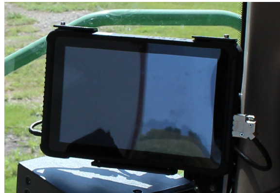
Fig. 2.17. Power and Serial Connections to Tablet Display.
