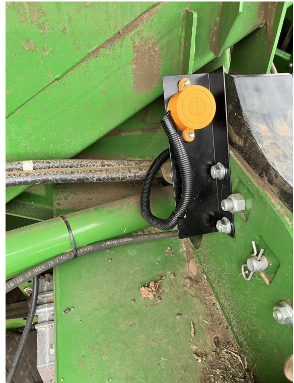
Fig. 2.9 Auger Sensor mounted under the unloading auger at the cradle.
