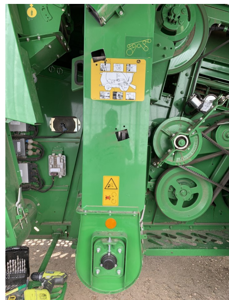
Fig. 2.3. Clean Grain elevator cut outs..
