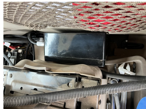
Fig. 2.8 NIR Spectrometer Box fitted behind the drivers seat.
