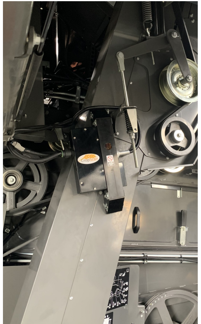
Fig. 1.2 Remote Sample Head mounted to the Clean Grain Elevator
