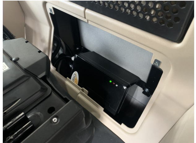
Fig. 2.6. NIR Spectrometer Box fitted to back wall.
