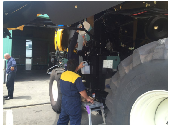
Figure 4.5. Pouring a sample through the CropScan sample head.
