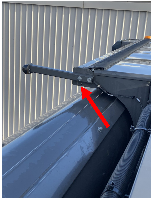
Fig. 2.9 Auger Sensor mounted to the Grain Tank chassis
