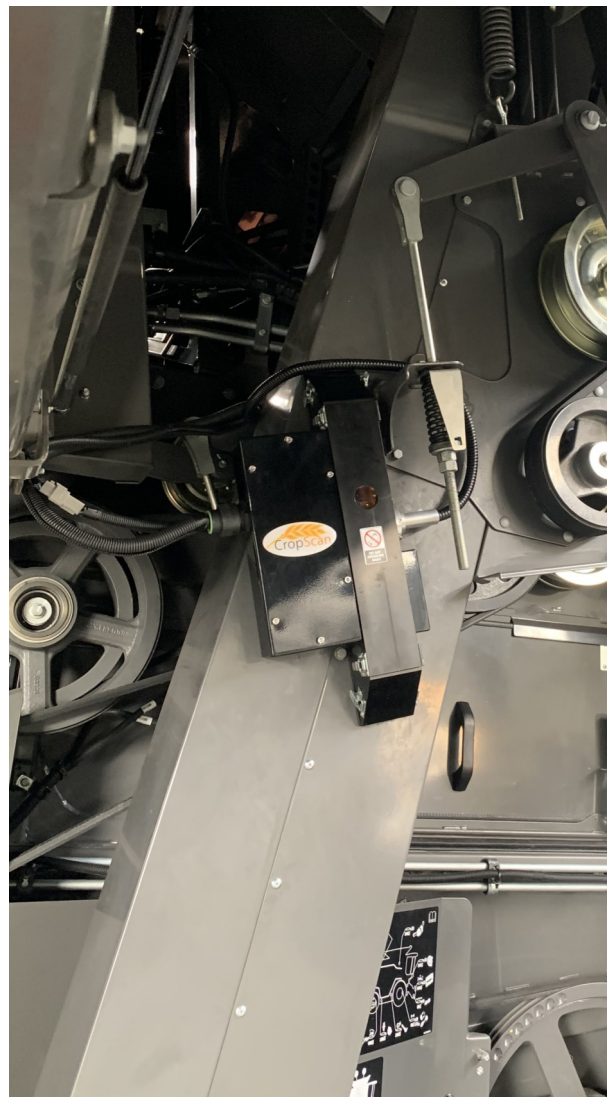
Fig. 2.5 Remote Sample Head installation .
