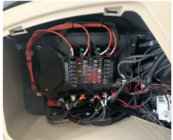
Fig. 2.15 Cabin Fuse access panel
