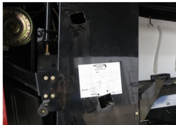
Fig. 2.3. Clean Grain elevator cut outs..
