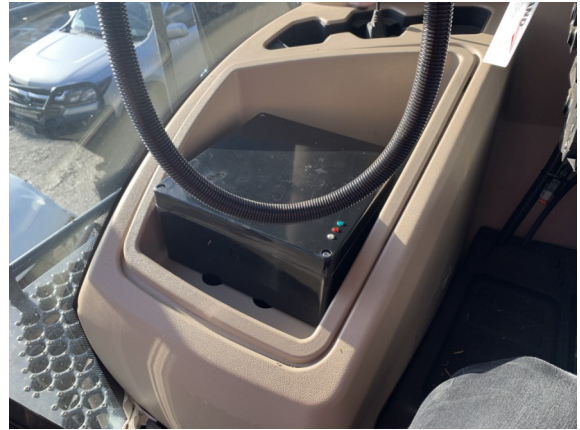
Fig. 2.8 NIR Spectrometer Box can be fitted to the centre console
