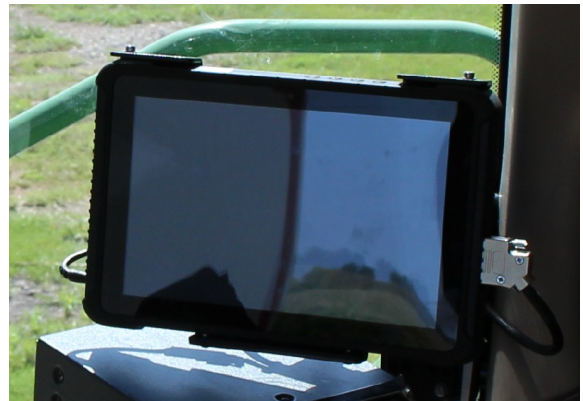
Fig. 2.11. CROPSCAN DISPLAY with power and serial connections.
