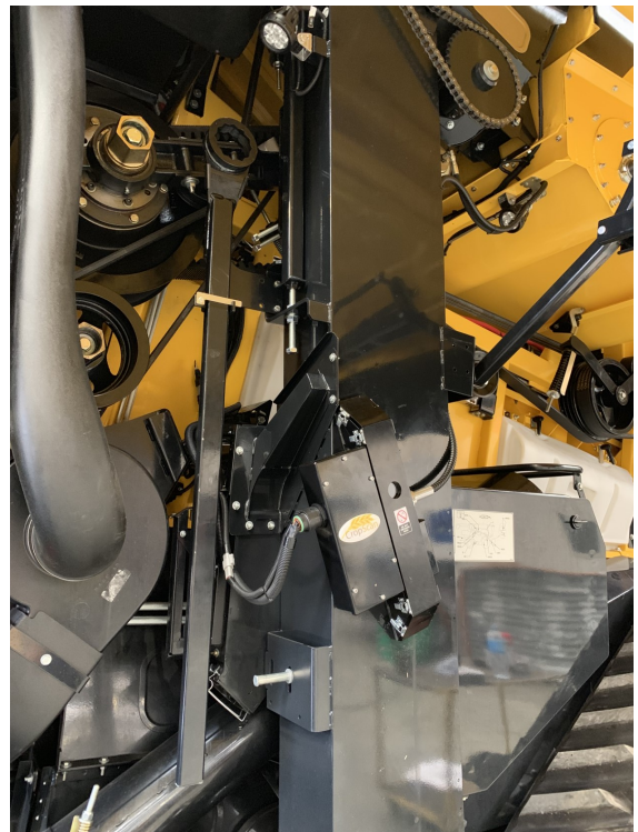
Figure 1-2. Remote Sample Head mounted to the Clean Grain Elevator
