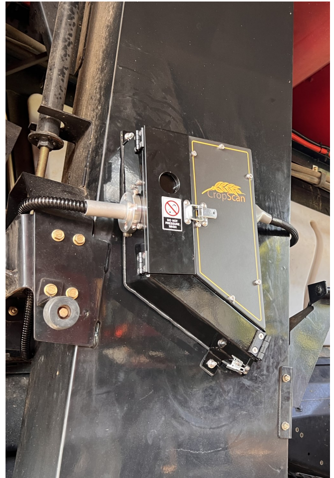
Figure 1.2 CropScan 4000VT On Combine Sample Head mounted to the Clean Grain Elevator.
