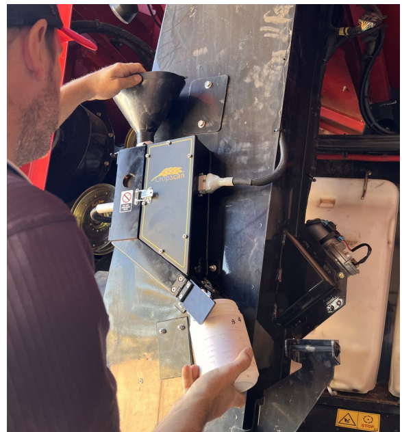
Figure 5.12 Auto Calibration Sample pouring
