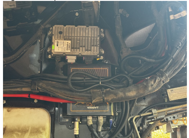
Figure 2.7. NIR Spectrometer installation mounting
