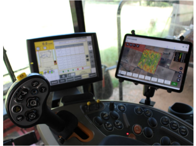
Figure 3.5 Case IH Cabin Layout optional Tablet Mounting.
