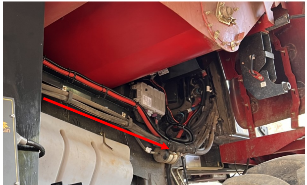
Figure 2.10 Sample Head Cable routing.
