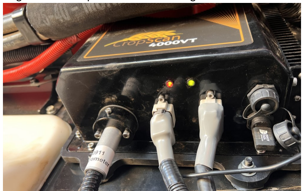
Figure 2.11 NIR Spectrometer connections.
