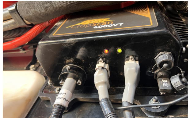
Figure 2.14 Spectrometer Cable connections.
