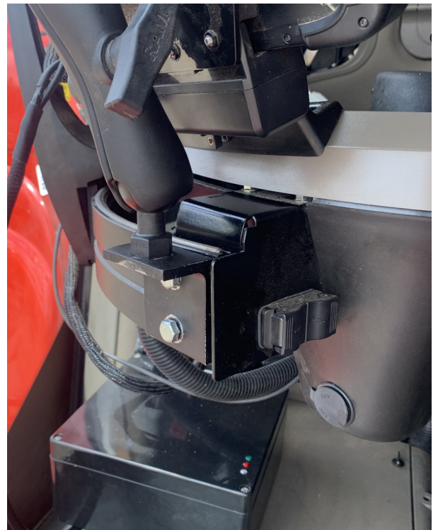
Figure 3.6 Optional Tablet Display bracket installation.
