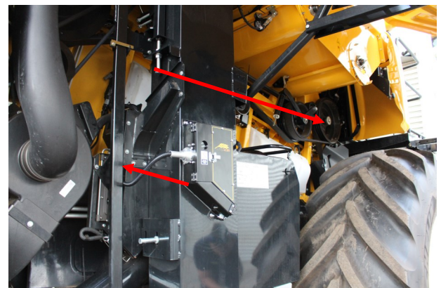
Figure 2.10 Sample Head Cable routing.
