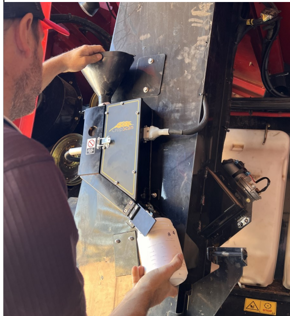
Figure 5.12 Auto Calibration Sample pouring
