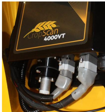
Figure 2.14 Spectrometer Cable connections.
