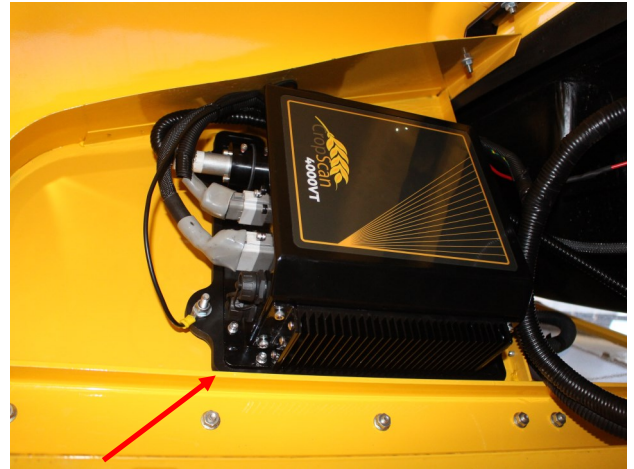
Figure 2.6. NIR Spectrometer attach studs.
