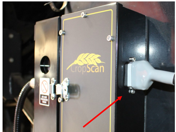
Figure 2.9 Sample Head - Power Cable connection.
