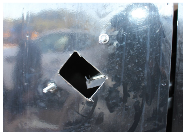
Figure 2.3 M6 Press Studs installed to the clean grain elevator.
