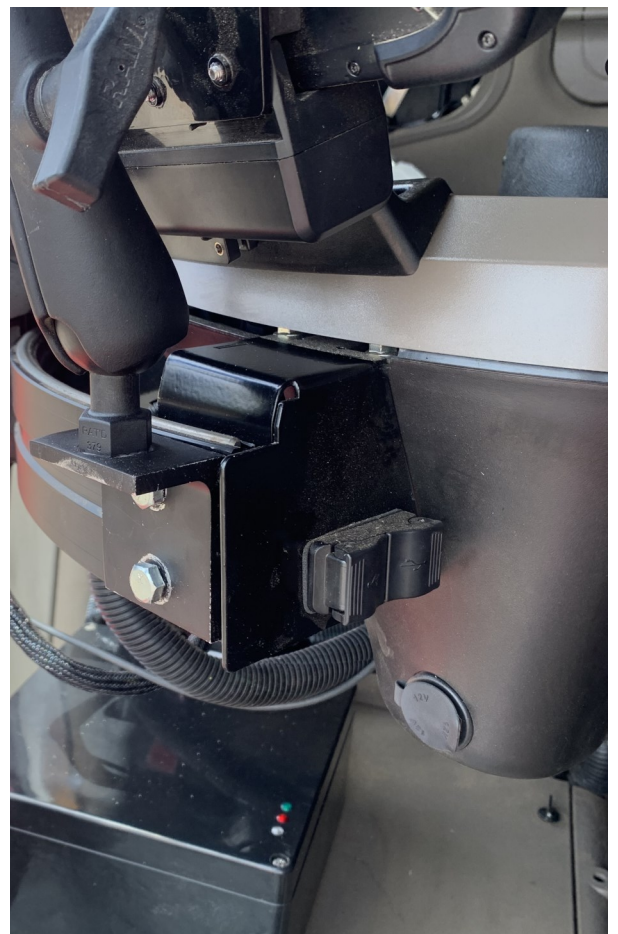
Figure 3.6 Optional Tablet Display bracket installation.
