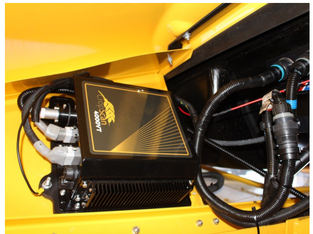
Figure 2.7. NIR Spectrometer installation mounting
