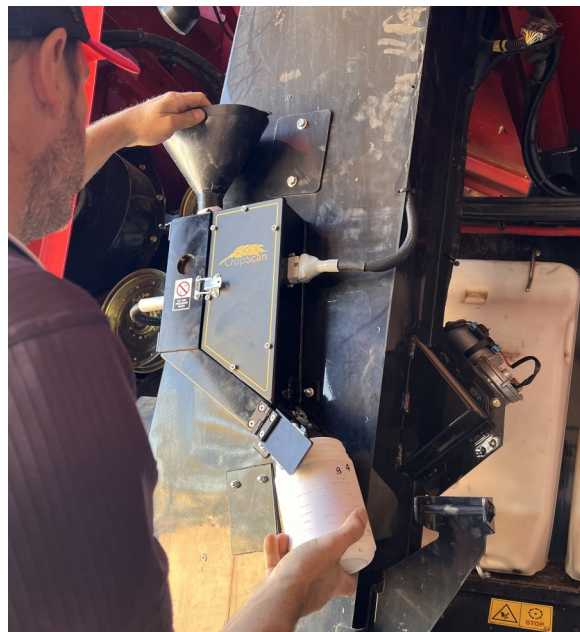
Figure 5.12 Auto Calibration Sample pouring
