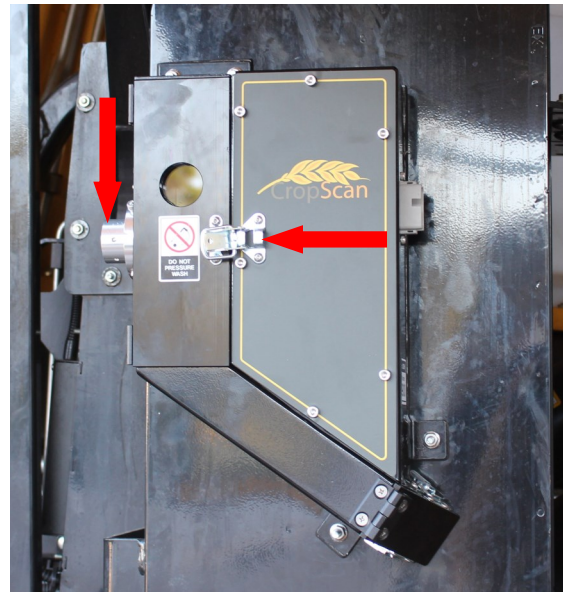
Figure 2.1 Sample Head Daily inspection points.
