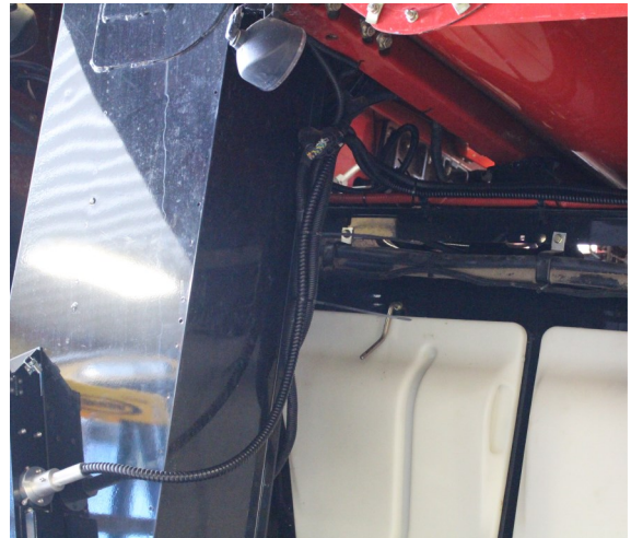
Figure 2.19. Sample Head and Fibre Optic Cable Run.
