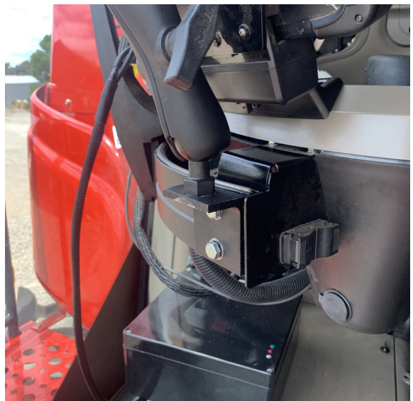
Figure 2.14. Display rail mounting position.
