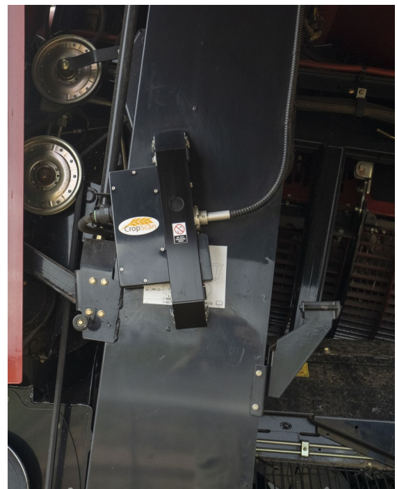
Figure 2.6 Sample Head installation.
