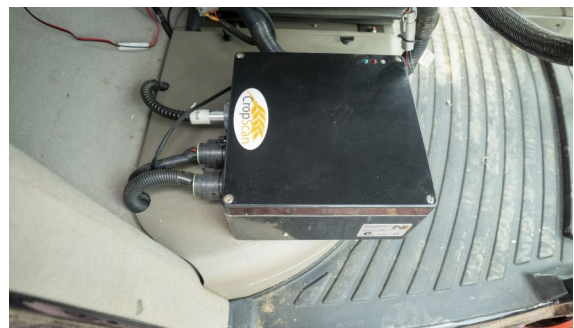
Figure 2.8 NIR Spectrometer Box fitted UCM Panel.
