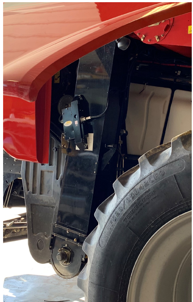
Figure 1.2 Sample Head mounted to the Clean Grain Elevator.
