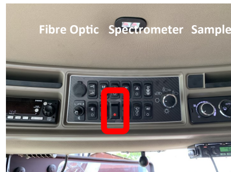
Figure 2.23, Spectrometer Power Switch installation
