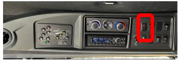
Figure 2.23, Spectrometer Power Switch installation
