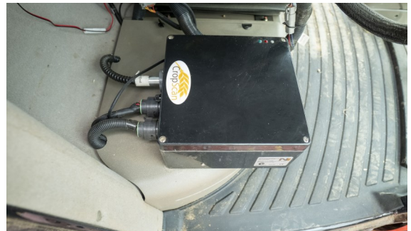
Figure 2.8 NIR Spectrometer Box fitted UCM Panel.
