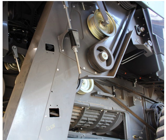
Figure 2.3. Clean Grain elevator Inlet and Outlet cut outs.
