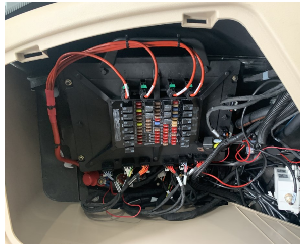
Figure. 2.17 Cabin Fuse access panel
