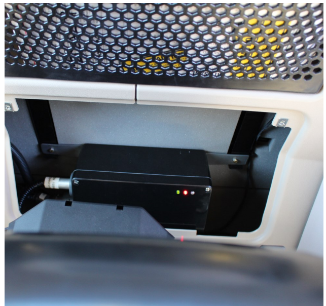
Figure. 2.7. NIR Spectrometer Mounting brace.
