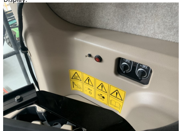
Figure. 2.20. ON/OFF Switch installation.
