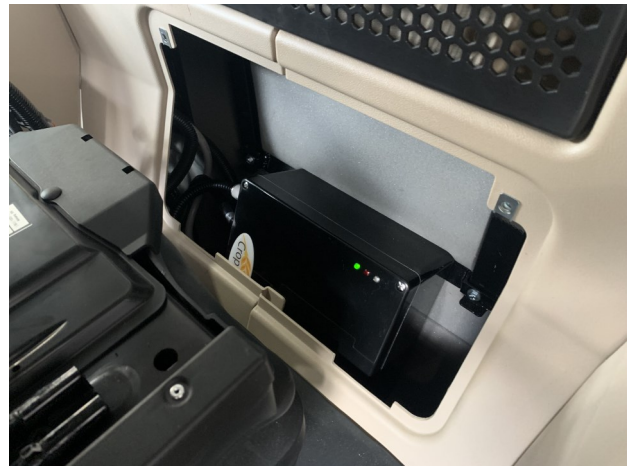
Figure. 2.6. NIR Spectrometer Box fitted to back wall.
