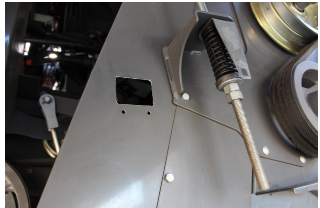
Figure 2.2. Clean Grain Elevator. Top Inlet Cutout and Hole.
