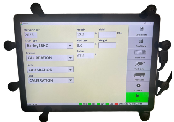
Figure. 2.13. CropScan Surface Go Tablet with power and USB Connections.
