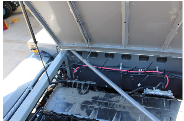
Figure. 2.8 Auger Sensor wiring routing.
